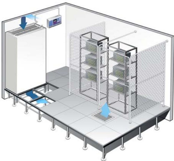
Illustration 2: Smoke detection at the CRAC return air grille.
